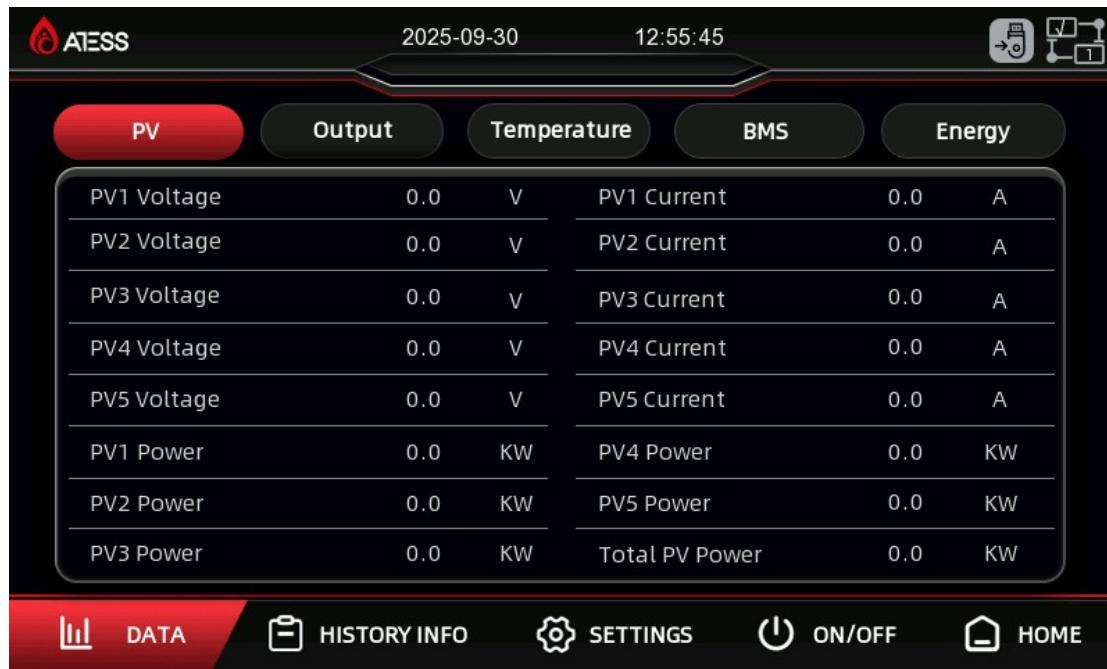
3.2 Measure whether the output voltages (points 5 and 6) match the values displayed on the screen.
