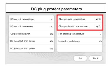
b.Gun temperature too high: This situation may indicate that there is overheating inside the gun head. Please suspend the use of the charger and further investigate.
