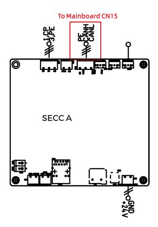
(2)Check SECC status: When SECC is working normally, there should be two lights, one constant and the other flashing. If there is no indicator light working, it indicates that SECC is not wkring. You can try to check if the power supply(CN1, 24V) is normal or replace the SECC board.
