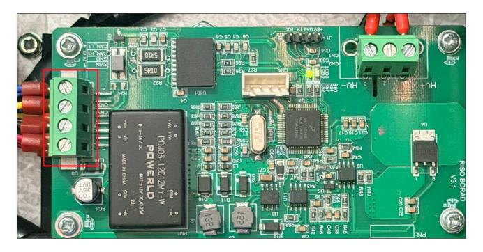
(2) If the charger still in fault after replacing the insulation detection board, it is necessary to consider the insulation of the entire charging circuit. First, check whether the gun cable is damaged, and then change a different vehicle for testing.
