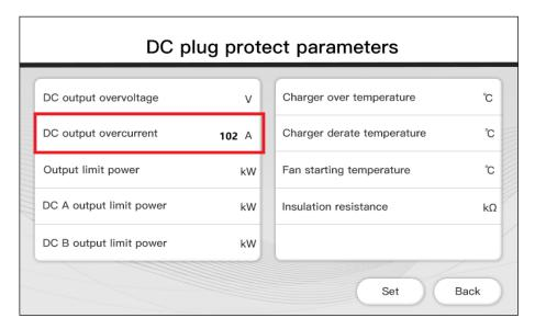
(3)Check the actual output current: Observe the actual output current value on the screen and use a clamp current meter to measure the actual output current. If there is a significant difference, it is a problem with the current sampling device. DC chargers usually use an electric meter to sample the current, which can check the shunt ratio of the electric meter parameters. For example, if two splitters are installed at the output end, the ratio parameter is set to 200.
