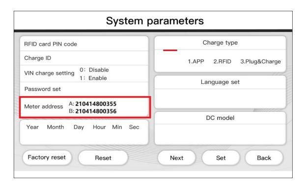
(2)Check communication cable: The communication between the electricity meter and the motherboard adopts 485 communication. The 485 communication line consists of two communication lines, namely A and B. The A and B lines between the electricity meter and the motherboard need to correspond one-to-one.
