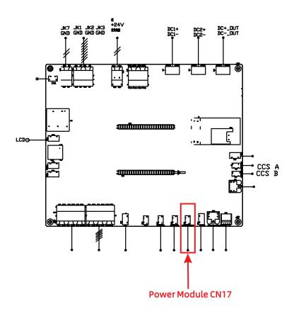
(2)Check power module runing light: When the fault occurs, please check the power module operation indicator light. If the operation indicator light goes out, it means that the power module is not powered and further investigation is needed to check the contactors between the power supply and the power module.
