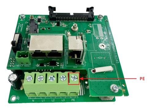
(2) Check the power supply: If the PE cable is tight but still give a PE fault, please search for relevant personnel to investigate the cause of external wiring.
