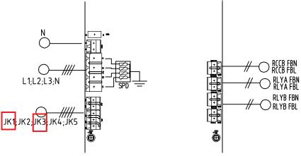
(3) Check relay: If the relay does not make a suction sound when starting to charge, or makes a sound during the charging process, it is considered that the relay itself is damaged and should be replaced.
