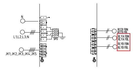
(2) Check relay drive circuit: Check if the relay drive signal voltage is normal at the beginning of charging. If the voltage are 0V, then it's a PCB issue, please replace.
