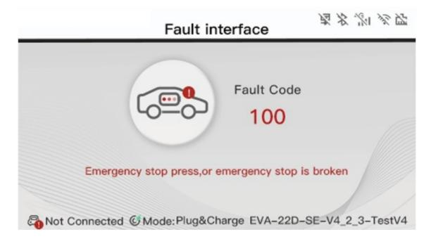
(3) Equipment Status: Charging stop and into fault status.
