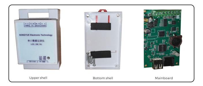
As shown in the figure above, a datalogger can be divided into three parts: the upper shell, the bottom shell, and the mainboard. Due to the different internal spaces of different EV Chargers, you can remove the protective shells and use only the mainboard for placement. In this case, please avoid metal contact with the mainboard.
