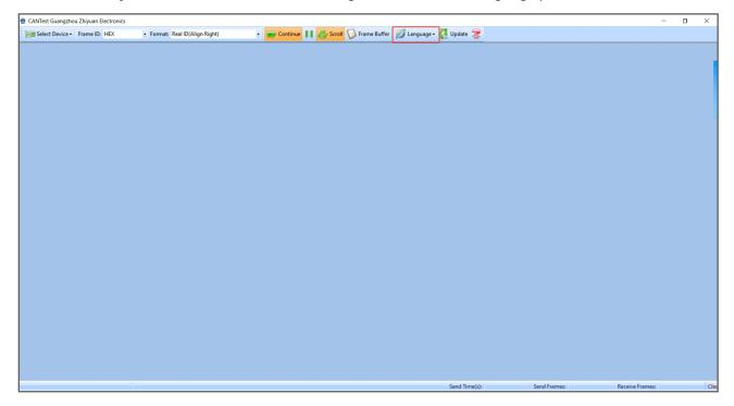
Click on the select device in the upper left corner and choose the CAN model to use. Generally, we only need to select USBCAN1. If you are using another brand of CAN box, you need to select the corresponding model.
