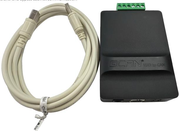
Firstly, connect the L and H on the CAN box to the CANA interface of the DSP or battery. Be careful not to reverse the connection. Generally, there are 2 adjustable resistance switches on the CAN box with a resistance value of 120 ohms, which do not need to be set under normal circumstances.
