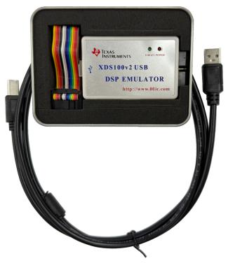
As shown in the figure, connect the computer and DSP through an emulator. It should be noted that during the update, the DSP board needs to be powered on, which means keeping the inverter's battery breaker on and other circuit breakers off. At the same time. The inverter needs to be in a fault state.
