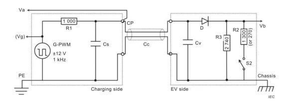
G-PWM PWM signal generator for pilot function
