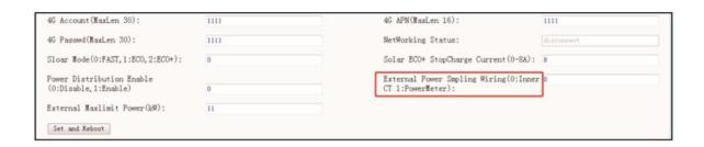
(4) Set the maximum power import value in the field of External Max Limit Power(kW). To avoid accidental tripping of the main breaker, it is suggested to set this parameter slightly lower than the maximum supply power of the property. e.g., the max supply power from the grid is 15kW, you can set the max power import to 13kW or 14kW.
