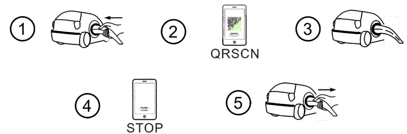
APP/RFID mode operation process flow
