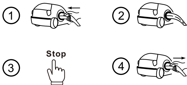
Plug&Charge mode operation process flow
