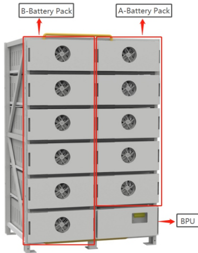
Figure-15 Installation position diagram of the battery and the BPU (picture is for reference only)
