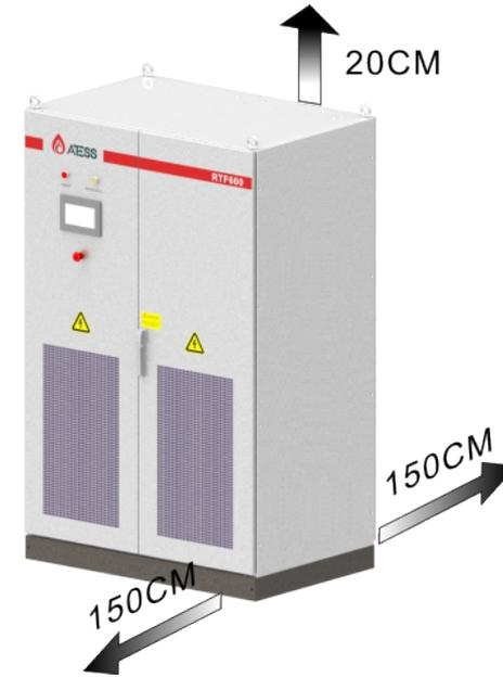
The front of the RTF installation position should provide a clearance of more than 1.5m, while the back and top should have clearances exceeding 1.5m and 0.2m respectively, in order to facilitate installation, efficient heat dissipation, and convenient maintenance.
