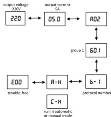
Figure 6 Key operation schematic
