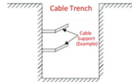
The design and construction of cable communication systems are typically carried out by the construction party in accordance with relevant standards, taking into consideration the weight and size of the equipment. It is essential to ensure proper electrical connections between cable trenches as well as between cable trenches and ground electrodes.
