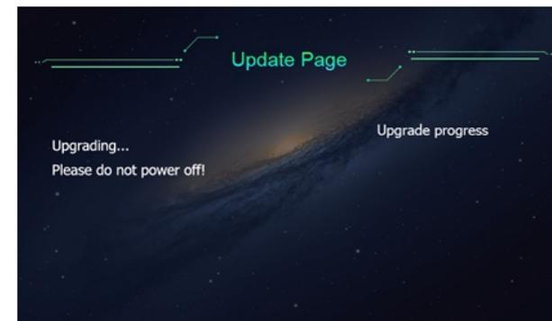
This interface will appear when you do a code upgrade. When the burning is complete, it will exit the screen and re-enter the main screen. In the interface state, to ensure the normal power supply of the machine, otherwise it will lead to burning failure. If the burning fails, it is necessary to re-power the burning.
