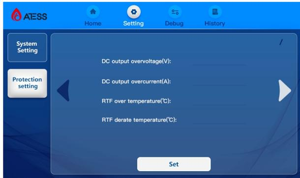
**DC outout overvoltage(V)** : DC overvoltage protection point. The maximum value is 1000V. It is generally set to the total voltage corresponding to the battery overvoltage protection.
