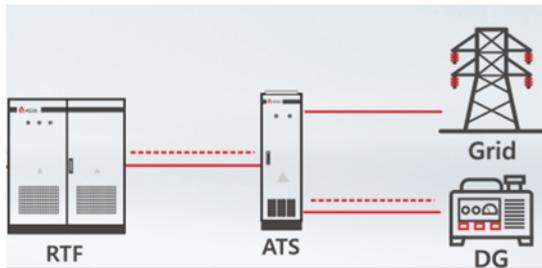
3. There are three circuit breakers inside the ATS, one is the BYPASS switch, and the other two are the GRID switch and the GEN switch. Pay attention to the cabinet label, do not connect to the wrong position, and pay attention to the three-phase phase sequence. Otherwise, the system cannot run normally.
