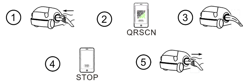
APP/RFID mode operation process flow
