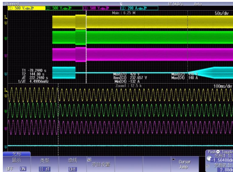
Response to utility recovery over voltage level 2
