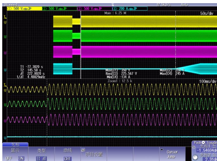
Response to utility recovery under voltage level 2
