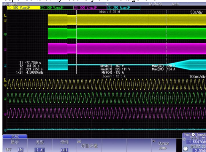
Response to utility recovery under voltage level 1
