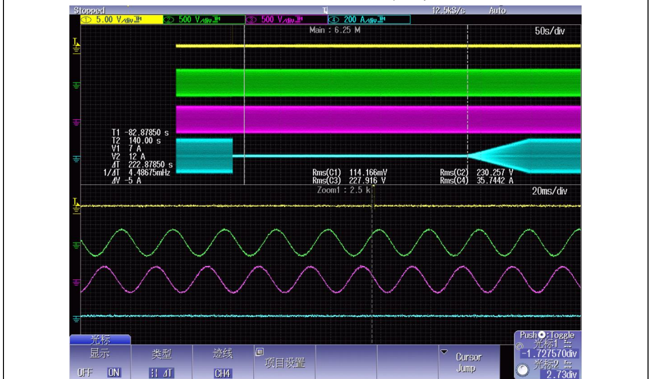
Reconnection after Over Frequency
