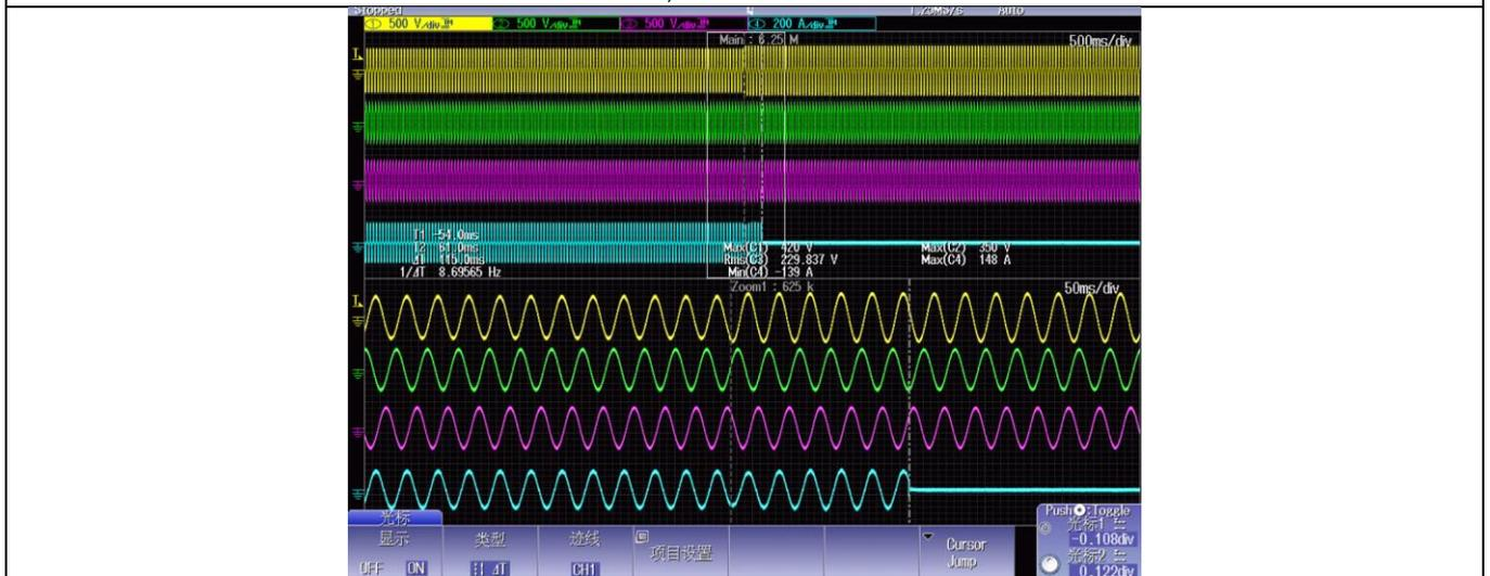
$V \geq 120\%$ ,  $L1 = 264\text{ V}$ ,  $L2 = L3 = 220\text{ V}$
