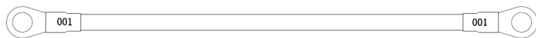
Figure 6-3 Schematic diagram of the series DC cable (picture is for reference only)
